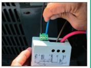
10] Attach the blue wire(supplied) to the Start Winding on the SureStart green terminal connector.
