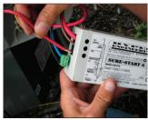
12] Attach the red wire (supplied) to the Active terminal on the SureStart.
